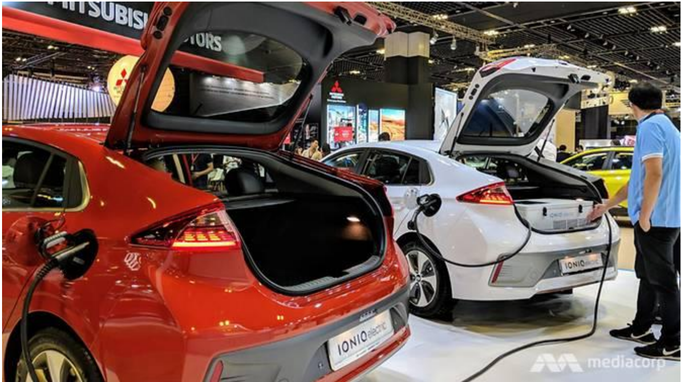
Demonstration of the Hyundai electric car by being charged by its 'emergency car'. (Photo: Christy Yip)
